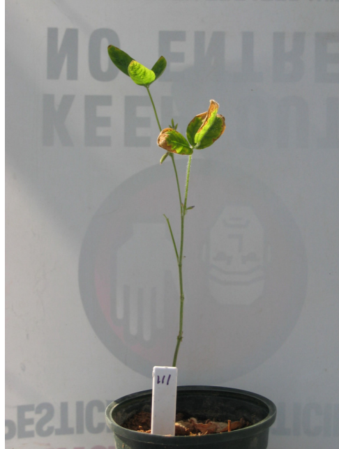
Figure 6. Soybean plant growing in acidic mine soil amended with 10% of CCP # 16. Note heavy stunting and complete loss/drop of lower leaves; typical of heavy soluble salt + B damage. Also note dropped leaves in pot that were totaled in yield estimates for Fig. 4.
