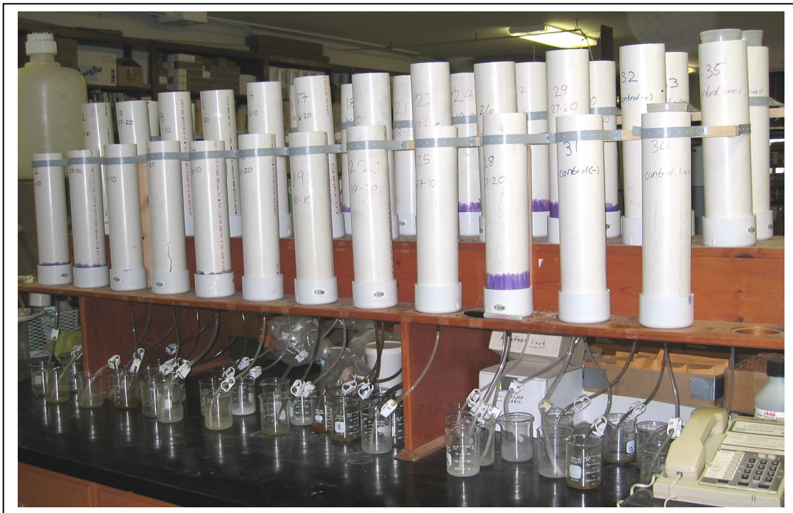
Figure 2. Photo of leaching column array in laboratory.
